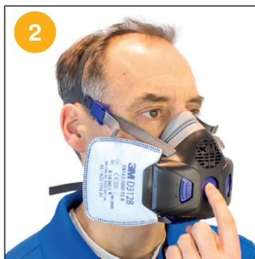
2. Lightly press the seal check button until you feel resistance. Hold the button in this position and inhale gently. If you feel the facepiece collapse slightly and pull closer to your face with no leaks between the face and facepiece, a proper seal has been obtained.
