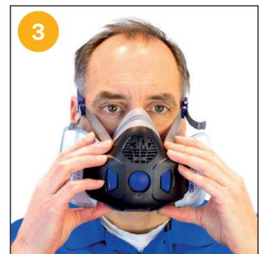
3. If faceseal air leakage is detected, reposition respirator on your face and/or readjust tension of the straps to eliminate air leakage. Repeat the user seal check until a proper seal is obtained.
