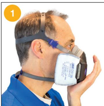
1. Cover the opening of the exhalation valve cover with your hand and exhale gently. If the facepiece bulges slightly and no air leaks are detected between your face and facepiece, a proper seal has been obtained.
